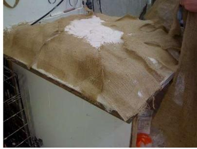
Once the mould was cured, the first plaster of parish casting was taken as a test cast.
